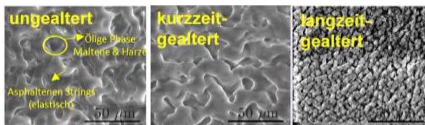
Figure 12: Bitumen under the electron microscope: (a) as delivered (unaged), (b) in the state of short-term ageing after mixing and paving, (c) in the state of long-term ageing after 10 years in the surface course (Blab & Hofko, 2012)
