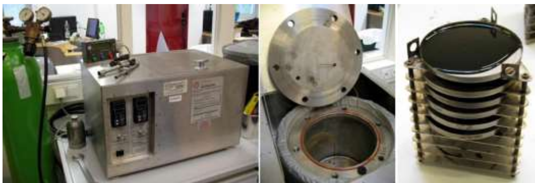
Figure 19: The apparatus for the PAV test: left: Pressure Aging Vessel, middle: Pressure vessel, right: Tray holder with filled trays (Hospodka, 2017)
