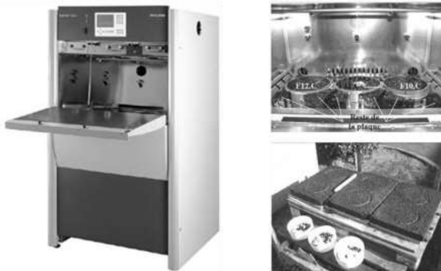
Figure 5: Ageing test: a) weatherometer for accelerated test; b) specimens artificially and naturally aged (Do, Kane, & Cerzo, 2014)
