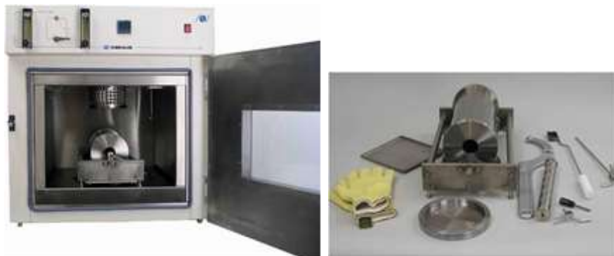
Figure 21: Accessory kit included with the NRC 210 for the Rotating Cylinder Ageing Test (RCAT) (Normallab France SAS, n.d.)
