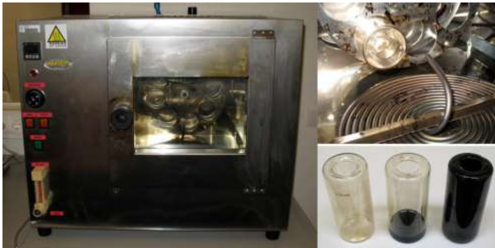
Figure 16: Apparatus for RTFOT: Rolling Thin Film Oven, top right: Air lance and vertical rotating drum, bottom right: RTFOT bottles (Hospodka, 2017)
