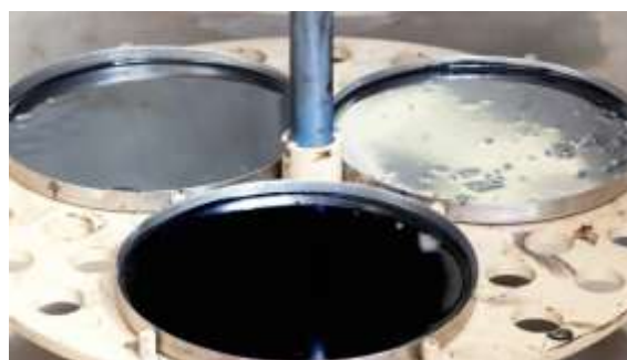
Figure 17: Performance of Thin Film Oven Test (TFOT) according to ÖNORM EN 12607-2 (Arbit, 2014)
