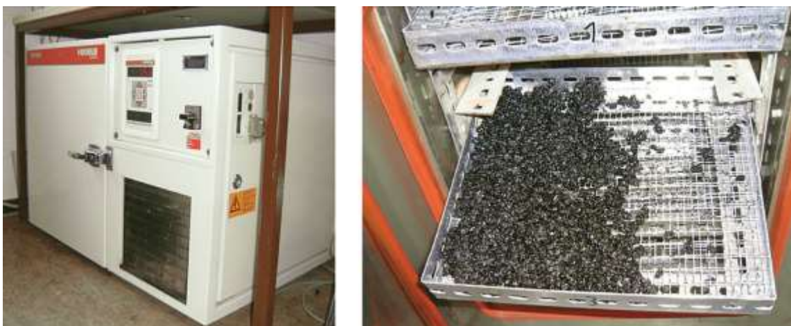
Figure 2: Material test cabinet and storage grate for Brunswick ageing (BSA) (Renken & Wistuba, 2018)
