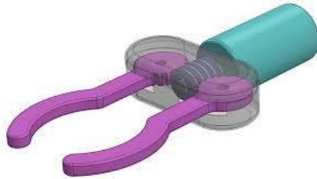
Figure 4: Gripper end-effector used for object handling (Fucile et al. , 2024)
