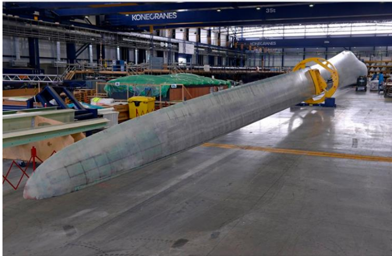
Figure 6: V164-80m long wind turbine blade (Milelr, 2023)
