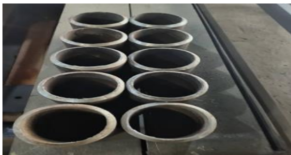
Figure 1: Bevel Pipe prepared for welding
