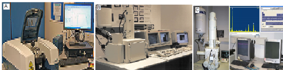
Figure 1: (a) Fourier transform infrared spectroscopy; (b) Scanning electron microscope; (c) Energy dispersive X-ray spectroscopy
