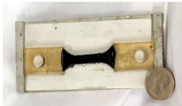
Figure 22. Direct Tension Tester - Mounted sample
