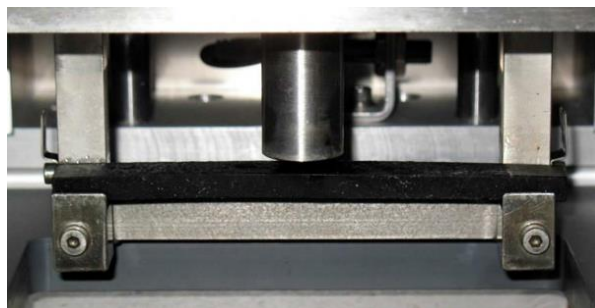
Figure 11. BBR test arrangement - bitumen beam
