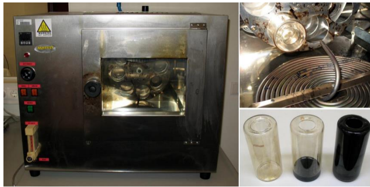
Figure 1. Apparatus for RTFOT: Rolling Thin Film Oven, top right: Air lance and vertical rotating drum, lower right: RTFOT bottles
