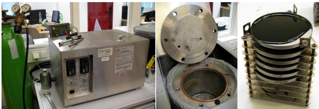
Figure 2. The apparatus for the PAV test: left: Pressure Aging Vessel, centre: Pressure vessel, right: Bowl holder with filled bowls
