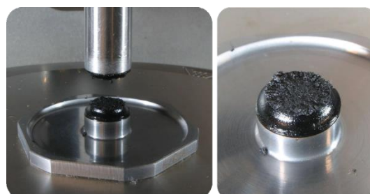
Figure 5. Clear cohesive fracture in the installed predetermined breaking point (specimen geometry with necking)
