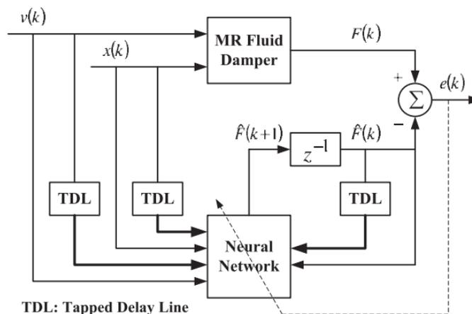
Figure 5: The scheme of identification for the MR fluid damper using the RNN model
