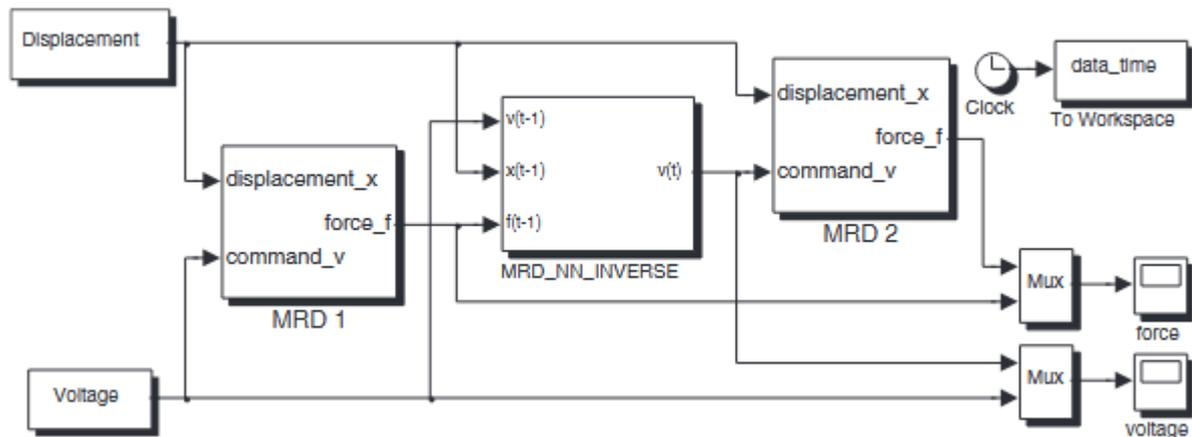
**Figure 8: The validation scheme for the inverse modeling with the FNN model for the MR damper**
