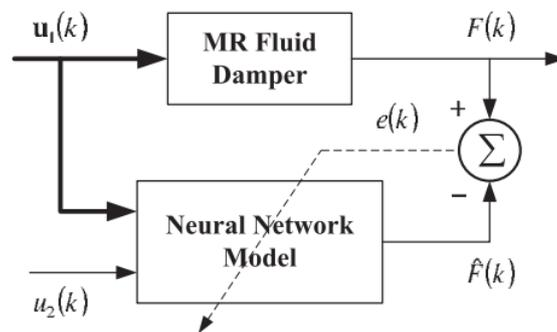
**Figure 3: The scheme of identification for the MR fluid damper using the neural network model**
