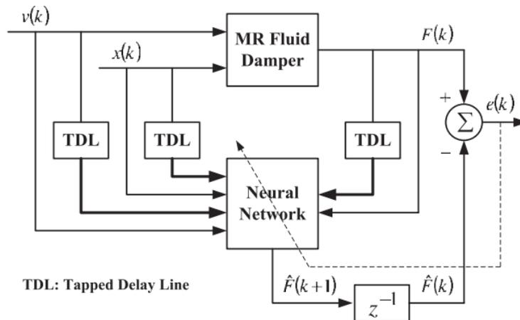
Figure 4: The scheme of identification for the MR fluid damper using the FNN model
