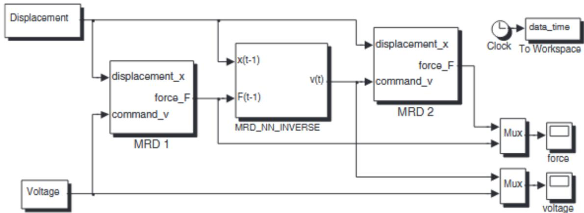
**Figure 9: The validation scheme for the inverse modeling with the RNN model for the MR damper**
