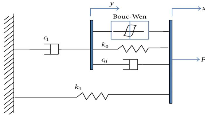
Figure 1: The dynamic model for the MR fluid damper
