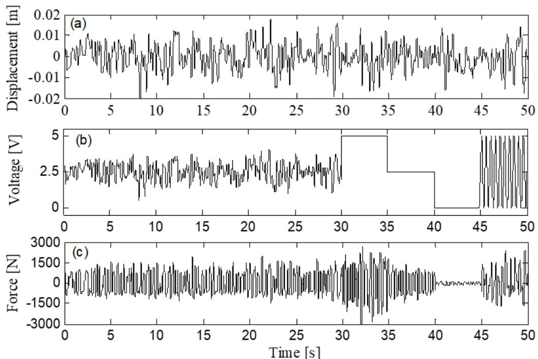
**Figure 2: The time history of training data sets for neural network models: (a) displacement; (b) command voltage; (c) damping force**
