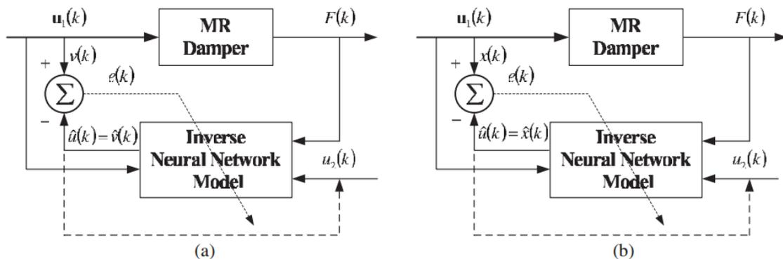
**Figure 6: The scheme of the inverse modeling for the MR fluid damper using neural networks: (a) force to command voltage model; (b) force to displacement model**
