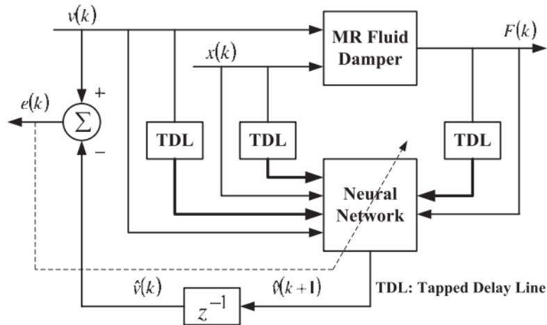
**Figure 7: The scheme of the FNN for modeling the inverse dynamics of the MR fluid damper**
