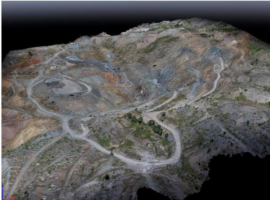
**Figure 6: The generated Point Cloud according to the RGB colors of the camera**
