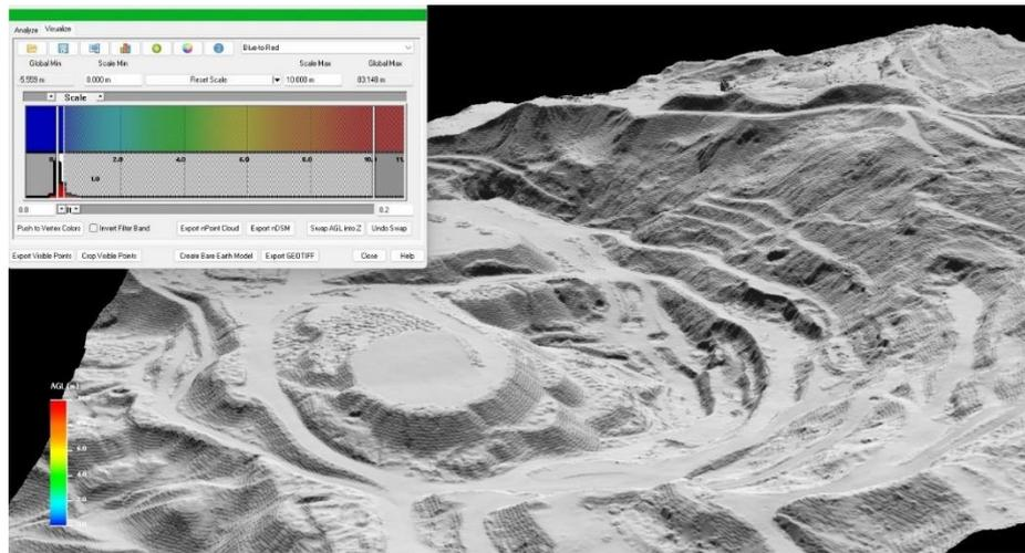
Figure 10: DTM generation in hillshade mode
