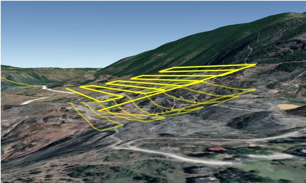
**Figure 5: 3D view of planned routes as well as live monitoring of flight execution**
