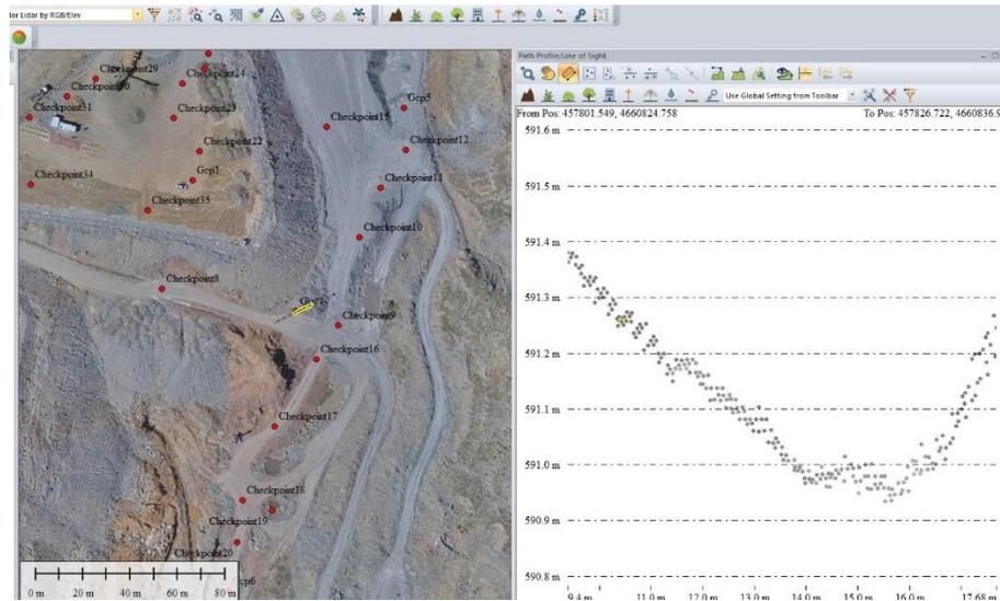
Figure 8: Visual control of the GCP position in a transverse profile
