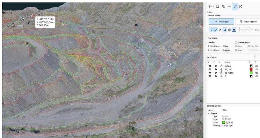
Figure 11: DTM generation in hillshade mode
