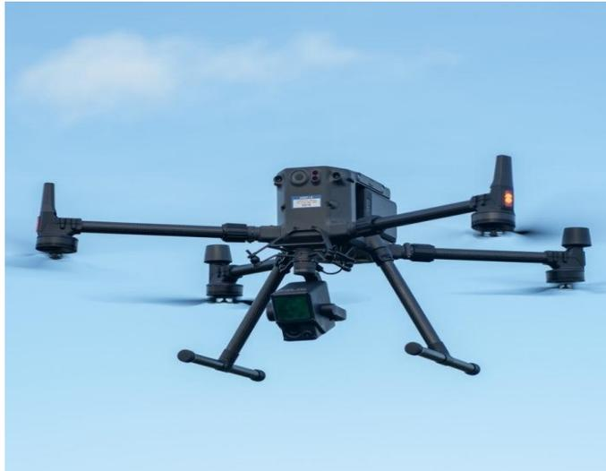
**Figure 2: DJI Matrice 300 RTK drone with Zenmuse L1 camera**
