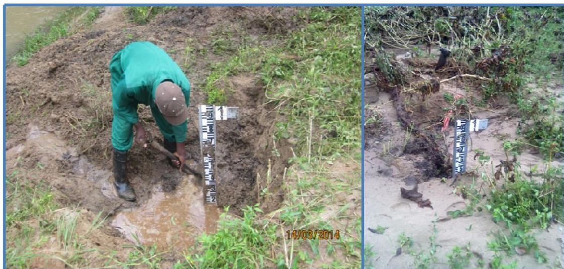
Figure 5: At the F24 Hydrological Station, gauge plates became clogged
