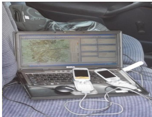
Figure 2: TEMS Measurement Tool used for Field gathering of RSS Data
