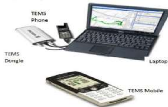
Figure 2: TEMS Measurement Tool used for Field gathering of RSSI Data
