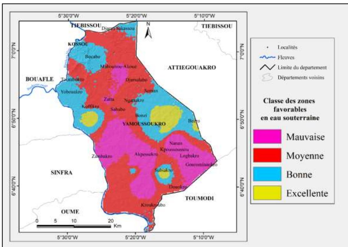
Figure 8: Spatial distribution of areas favourable to the installation of high-flow hydraulic boreholes
