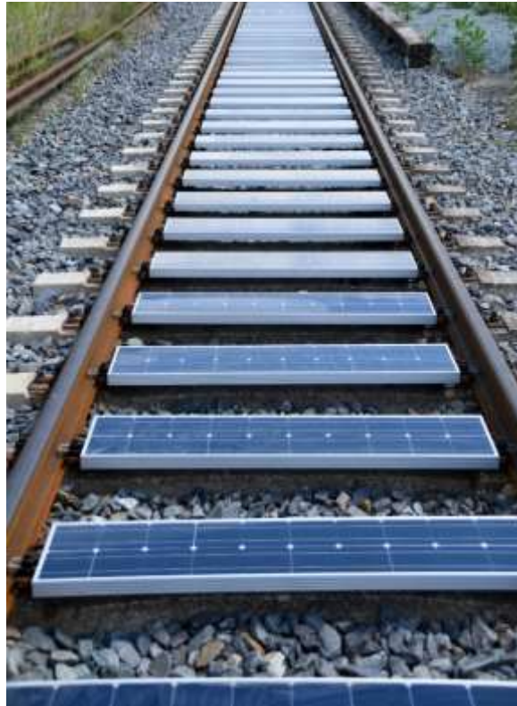
Figure 18: Bankset Energy is testing solar modules on railway sleepers at the DB test field. To do this, they use small modules that they mount individually on the sleepers (Koch, 2023)
