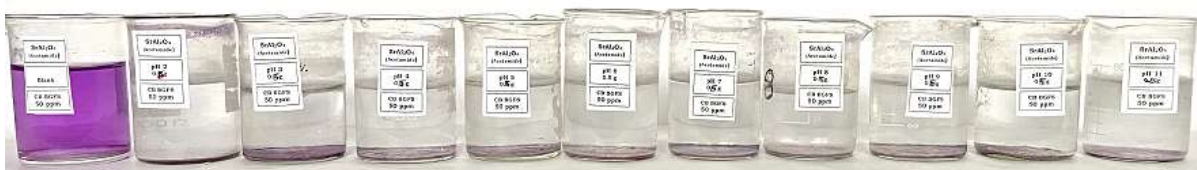
Photo 2: Effect of pH on Coralene Blue BGFS at 300 minutes 50ppm/L, pH=7, SrAl 2 O 4 (Acetamide)
