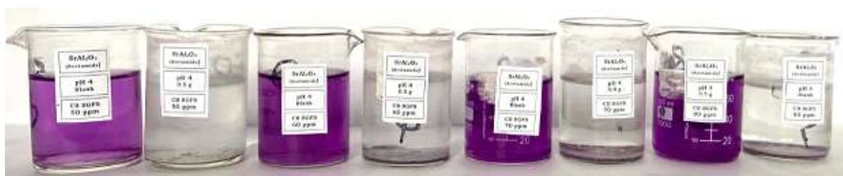
Photo 3: Effect of initial dye concentration on the photocatalytic degradation of Coralene Blue BGFS by \text{SrAl}_2\text{O}_4 (Acetamide) 50, 60, 70 & 80ppm pH=0.5g/4
